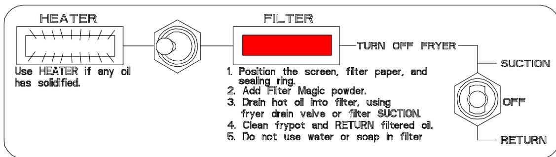
Use the filter heater for 20-30 minutes prior to filtering if solid shortening is filtered.
