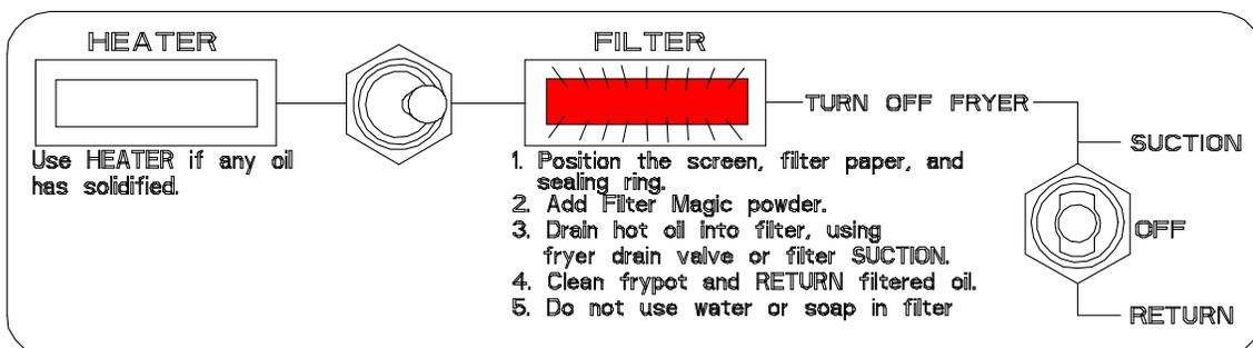
The Heater/Filter switch must be in the FILTER position before the filter pump can be operated. The red light will illuminate when the switch is properly positioned.
